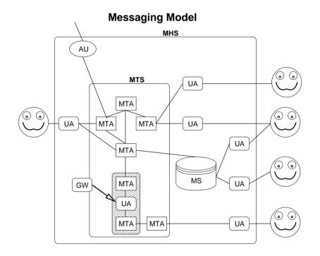
As can be seen, a user may use more than one UA, and a UA can be connected to more than one MTA.
