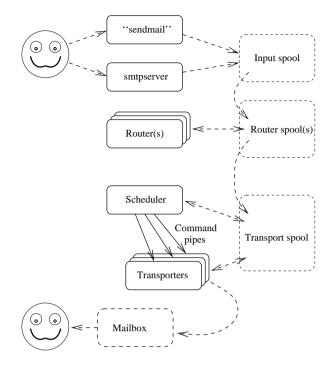
ZMailer is a multi-process mailer, using three daemon processes to manipulate messages. Used technologies are as simple as possible, e.g. while networking stuff is as advanced as possible (with fallbacks to simplest basic behaviour), some of other modern things (like threads) are not used in favor of simpler approaches
